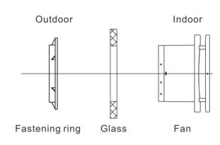
**Step 2:**Remove the fastening ring from fan.
