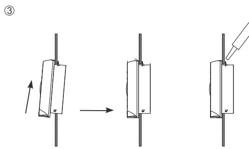
Insert the exhaust fan into the glass hole according to the drawing, rotate the main body to the normal position, and tighten the periphery with glass glue injection
