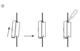
Insert the exhaust fan into the glass hole according to the drawing, rotate the main body to the normal position, and tighten the periphery with glass glue injection
