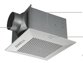
The fan casing is made of galvanized steel and the decorative front plate is made of ABS plastic and fitted with a filter.
